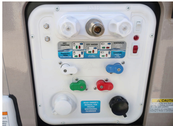
Water Center Panel in “Winterize” configuration (Panel located behind passenger rear door)
