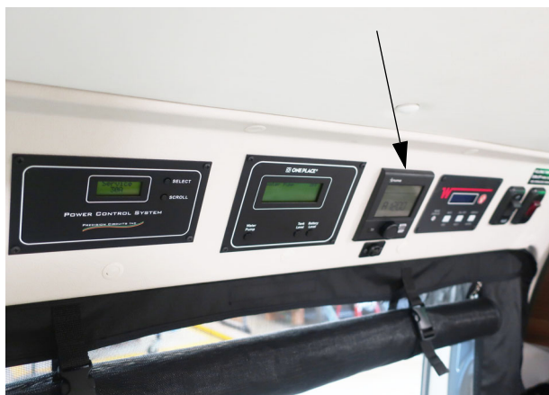
Water heater controls on Systems Monitor Panel *Model 59K shown -Typical View
