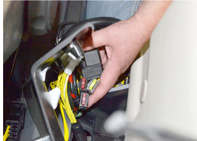
Trailer Plug Fuses (Located behind plastic panel on pillar behind passenger seat)
