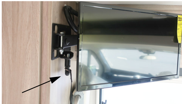
Grasp TV and disengage from the wall mounting bracket. -Typical View
