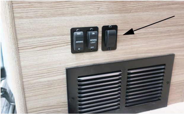
Accent LED Running Board Light Switch (Located near sliding entrance door) -Typical View
