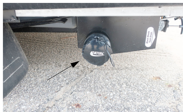
Sewage Drain Outlet (Located beneath motorhome) *Model 59K -Typical View
