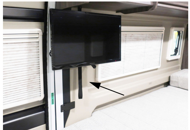
Pull straight down to release -Typical View
