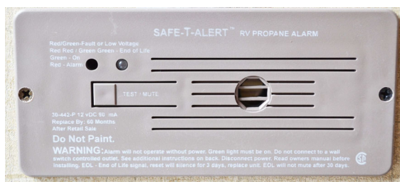
Propane Gas Leak Detector
