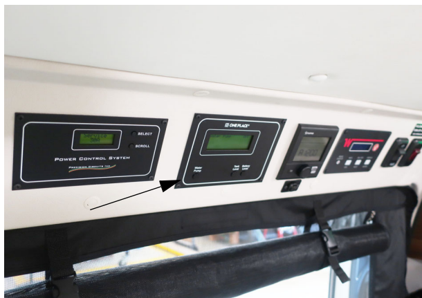
Water pump switch location on Systems Monitor Panel *Model 59K shown -Typical View
