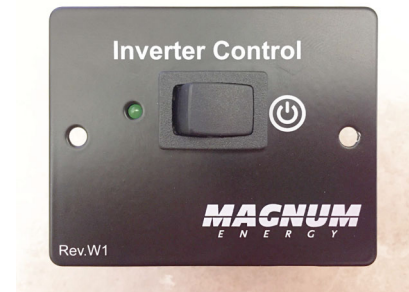
Inverter Control Panel (Located near monitor panel) -Typical View
