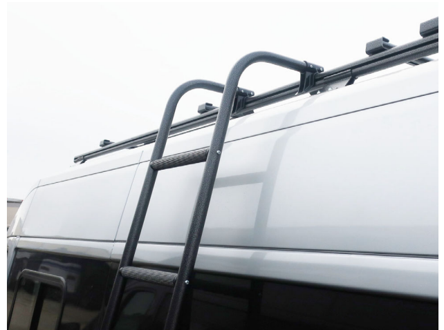
Shown with Ladder properly mounted on rail at driver side.
